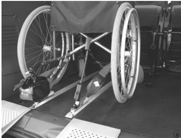
Figure 6 UNWIN overrun platform, assembled by Cebzon
